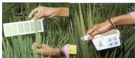
Leaf color chart (left) is found to be an inexpensive alternative to SPAD chlorophyll meter (right) for effective N top dressing
